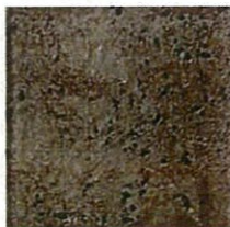
Salted concrete to retain industrial texture; with no art inlays
